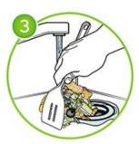
Feed the food waste into the disposer. Listen for the disposer to finish its work.
