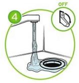
After grinding is complete, turn off the disposer and let the water run for a few seconds to flush the drain line.
